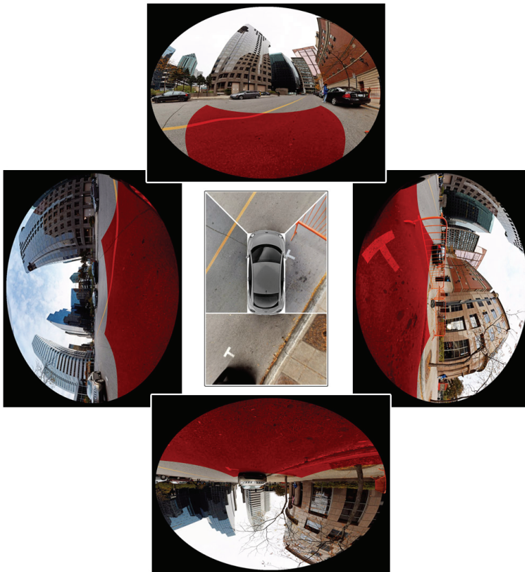
Fig. 31. View of area surrounding vehicle using four (4) panomorph lenses.
