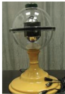
Fig. 8. Full sphere ODVS with back to back configuration
